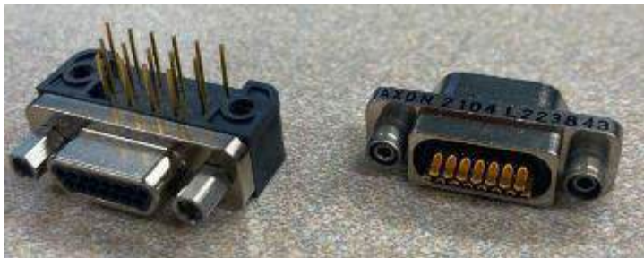
Non-magnetic (<20 nT) \mu -Dsub Connector
